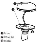
2. Screw on the receiver base to the stem first, making sure that the stem pipe does not protrude from the receiver base. This adds protection to the cable when pulling it through the pipe stem. In addition to this, de-burr the pipe edges to reduce cable abrasion. 3. Use electrical tape to secure the NMEA pigtail to the cable as shown.
